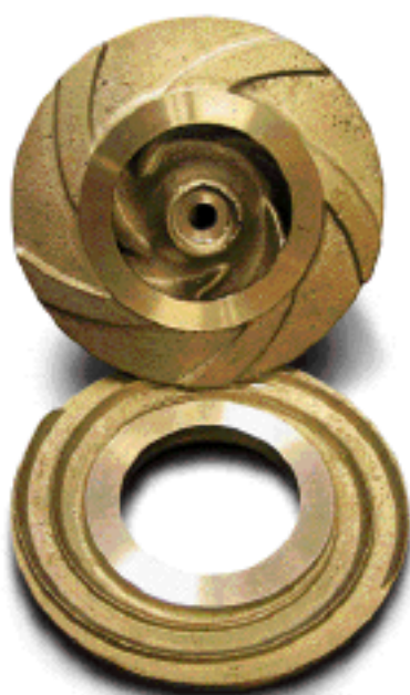
The back vanes (top) and spiral groove (bottom) ensure that only the finest particles reach the impeller neck, thus reducing wear and tear.
